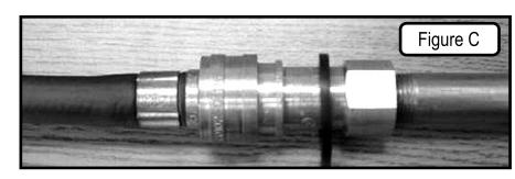
With proper assembly the gas hose cannot be removed without pushing the quick disconnect sleeve back. To disconnect, push the sleeve back and pull plug out of sleeve (this automatically shuts off gas).
